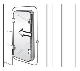
Press the light cover into the metal frame.
